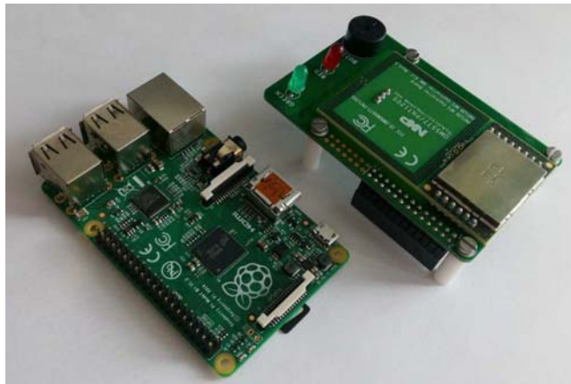
Figure 26: NFC Controller and Raspberry Pi Boards
