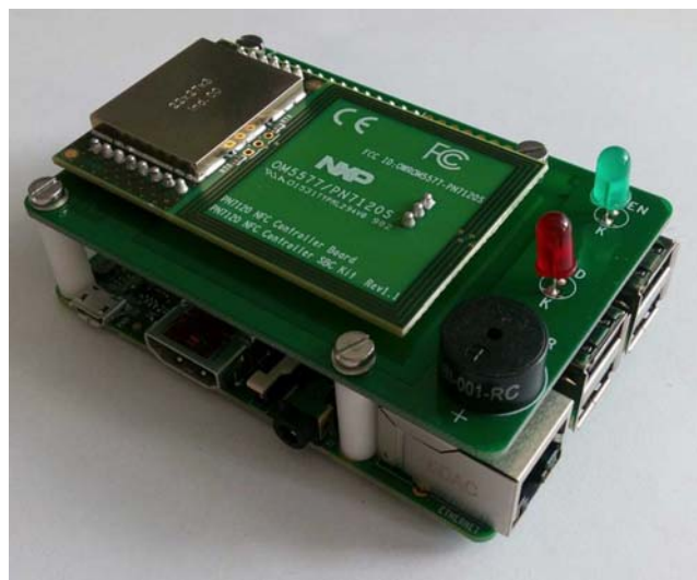
Figure 27: NFC Controller Board Mounted on Raspberry Pi Board
